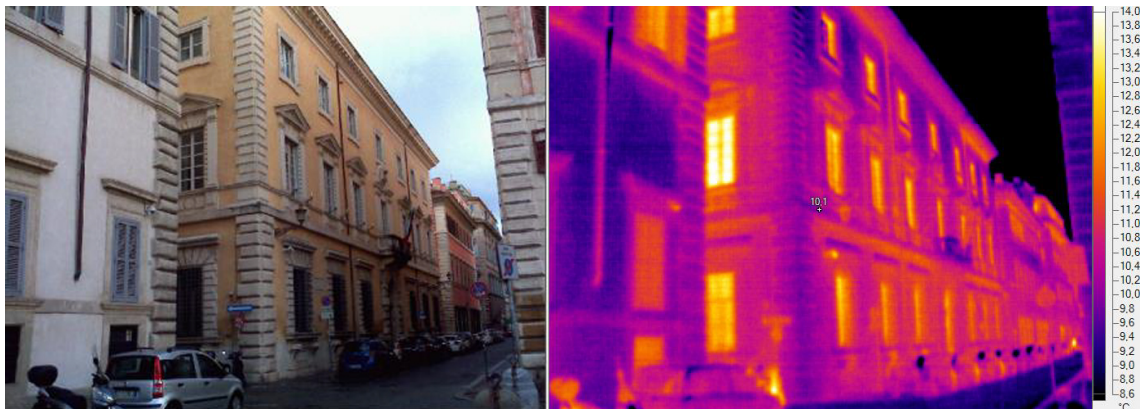
Photography and corresponding thermography analysis of the Italian case study Palazzo del Clementino – Maffei Borghese (BEN ISPC-CNR)
