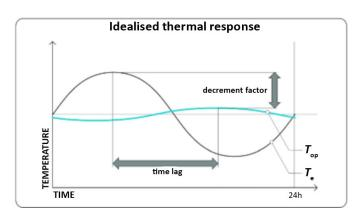
Fig. 34. Idealised thermal diurnal performance of extremely lightweight (top) and high mass (bottom) building. Te and Top correspond to outdoor and indoor temperature respectively. Source: Košir 2019.
