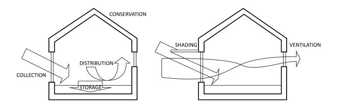
Fig. 32. Passive solar energy collector (left) and overheating avoidance (right) in temperate climates. Source: Norton, 2014.
