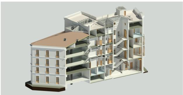
Fig. 9. Render view of the EE- HBIM model of the Spanish pilot building "Palacio de Calatayud" in Valencia.
