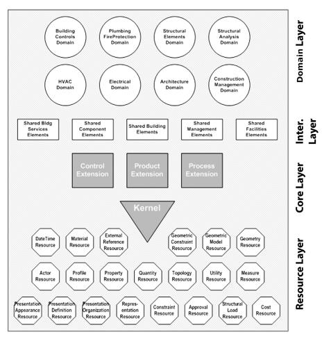
Fig. 29. IFC Data schema with four conceptual layers (buildingSMART 2020).
