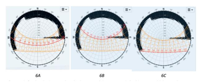
Fig. 21. Solar shading mask in the location of the case-study building in Bethlehem, where B: at summer solstice, C: at winter solstice. Created through the application: Source: https://drajmarsh.bitbucket.io/shading-box.html)
