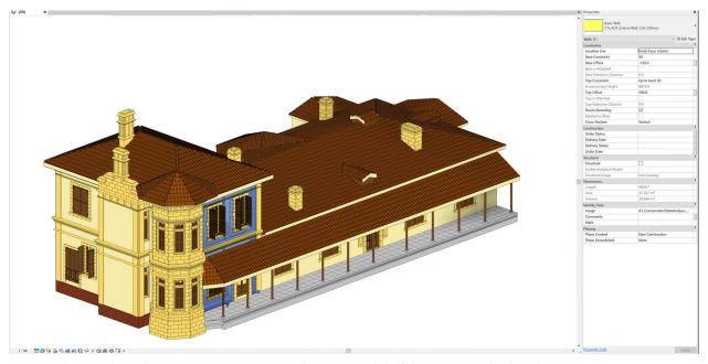
Fig. 10. Object selected to view its properties in the BIM model of the Cypriot pilot building.
