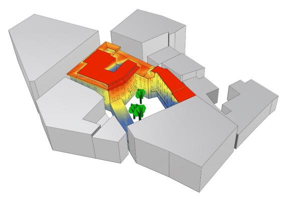
Fig. 5. Analysis of the sunshine duration on the façades of the Italian case study, to select the areas of minimum sunshine radiation to perform the Heat Flux meter analysis.
