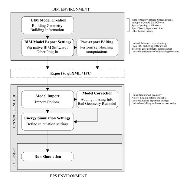
Fig. 26. Schematic representation of BIM to BPS Interoperability problem
