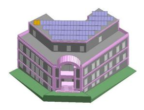
Fig. 14. Energy model of the Municipality of Tripoli showing the PV and SWH panels
