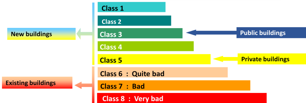
Fig.4: Scale of classification of buildings energy performance
