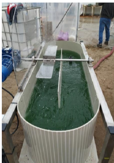
Figure 37. 200-litre capacity raceway-type reactor built within the framework of the MedArtSal subgrant programme at the Preciosa y Roqueta salina (Bay of Cadiz, Spain). It is made of polypropylene on a metal support so that its location can be changed. ©MedArtSal project
