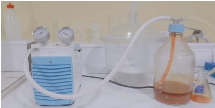
Figure 46. Device for D. salina carotenoids extraction by air bubbling at laboratory scale. ©SAIDA S.A.
