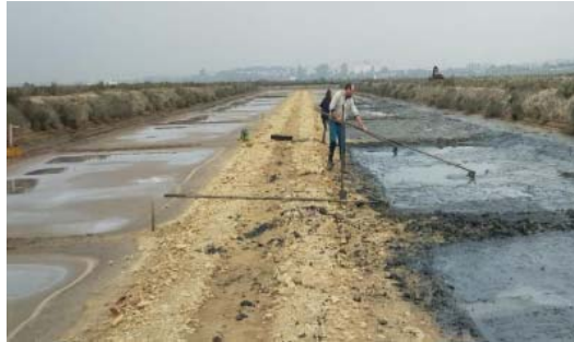
Figure 6. Salt workers cleaning the crystallisation ponds manually. ©SC-ISE UCA
