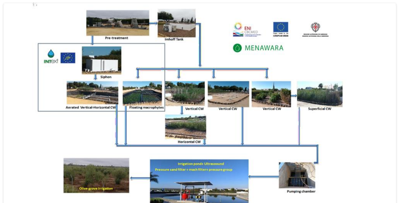
Figure 10. Schematic representation of the working configuration, including Pre-treatment, Imhoff Tank, reception and pumping chamber, storage pond and post-
