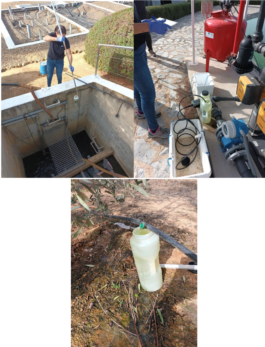
Figure 5. Illustration of AMAYA's staff sampling at the outlet of CWs, Filtration system and in the irrigation piping at the plot.
