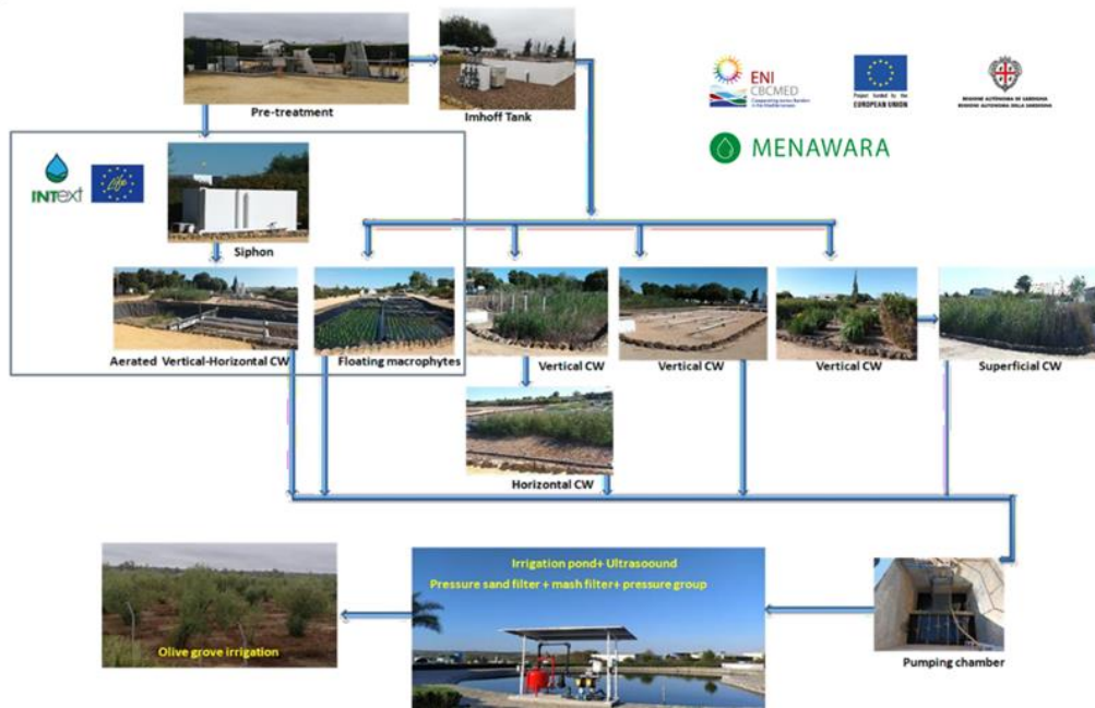
Figure 3. Schematic representation of the working configuration, including Pre-treatment, Imhoff Tank, reception and pumping chamber, storage pond and post-treatment train implemented in the MENAWARA project and plot for irrigation of olive groves experiences.
