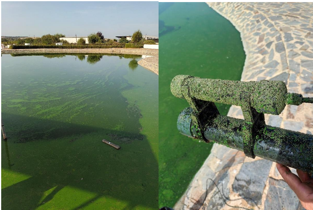
Figure 15. Illustration of algal bloom in the accumulation pond and fouling of the ultrasound equipment.
