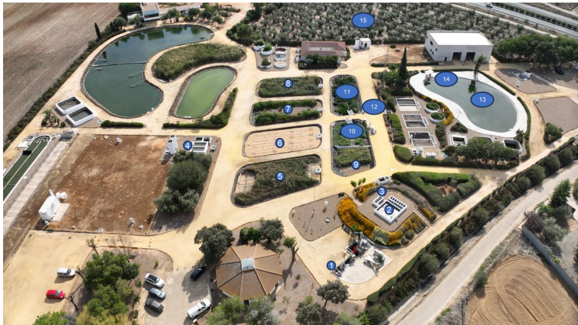
Figure 4. Aerial view of treatment units at Carrión de los Céspedes Experimental Center, Seville, Spain: 1- Pre-treatment; 2- Homogenization tank; 3- Distribution channels; 4- Imhoff Tank; 5- Vertical Subsurface CW-1; 6- Vertical Subsurface CW-2; 7- Vertical Subsurface CW-3; 8- Fre Water Surface CW; 9- Horizontal Subsurface CW; 10- Aerated vertical-horizontal CW; 11- Floating helophytes; 12- reception and distribution chamber; 13- Storage pond; 14- Post-treatment: ultrasound unit + automatic pressure sand filter + manual cleaning mesh filter + pressure group; 15- Olive grove plot.
