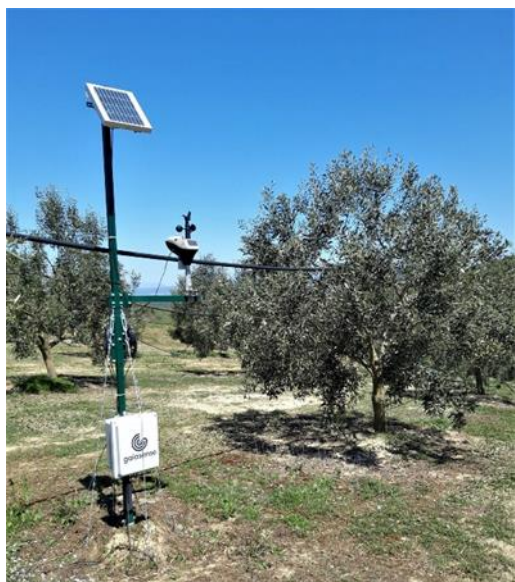
Image 1: A giasense agrometeorological station in an olive grove (by NEUROPUBLIC)
