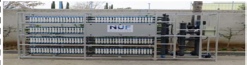
Industrial NUFILTER plants – modular, fully automated units for public swimming pools
