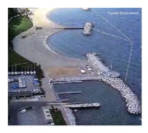
Figure 12 Groynes and breakwaters along the Greek coasts (Source: Discovering Happisburg).
