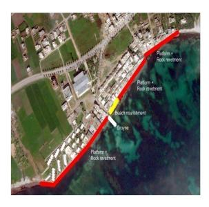
Figure 10 Combination of different protection works along the El Mamounia section in Kélibia (Tunisia), 2017.
